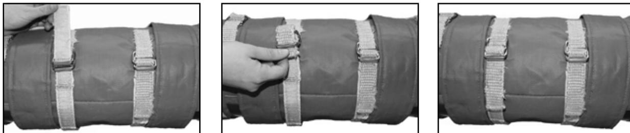
Ease of use is built into the design of the insulation jackets - they are lightweight, modular, and easy to handle so that employees can easily reinstall them on machines. The jackets use a strap and buckle system rather than hooks and wire - so no tools are ever necessary to secure them in place.
