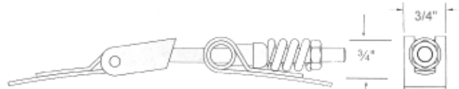
Fig. R: Quick Release Clamp Assembly with 1/4-20 bolt.
